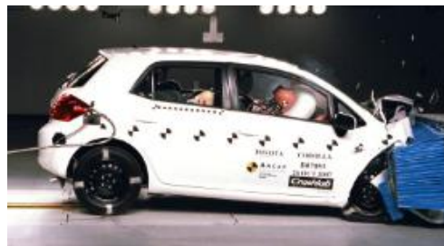
Offset crash test at 64km/hr
