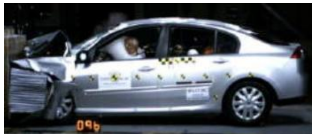
Offset crash test at 64km/hr
