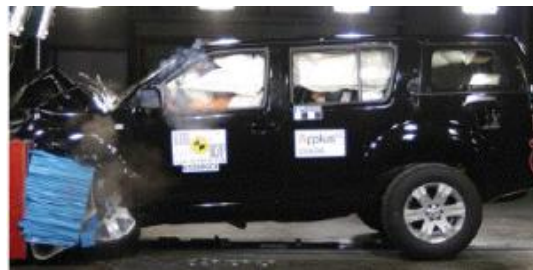
Offset crash test at 64km/hr
