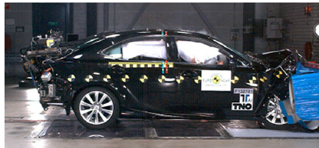
Frontal offset test at 64 km/h (Euro NCAP)
