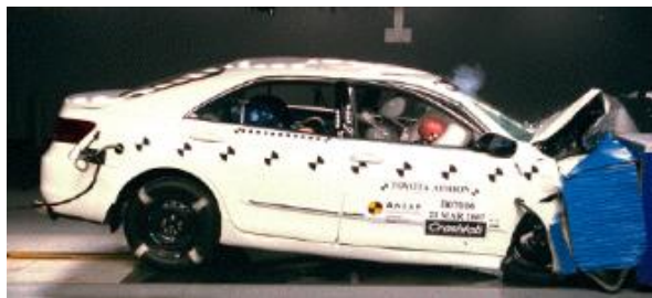
Offset crash test at 64km/hr
