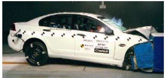
Offset crash test at 64km/hr
