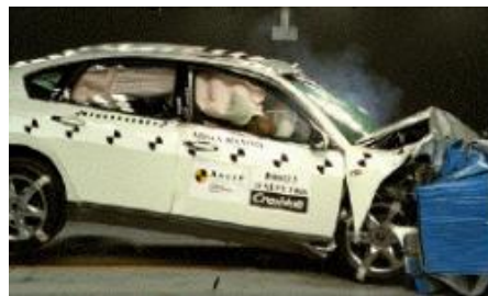
Offset crash test at 64km/hr
