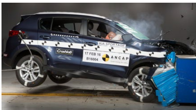
Frontal offset test at 64km/h
