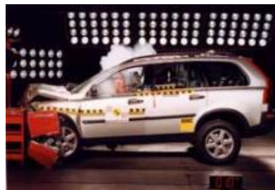
Offset crash test at 64km/hr
