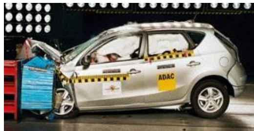
Offset crash test at 64km/hr
