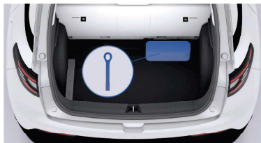
Rescue Traction Ring Storage Location
