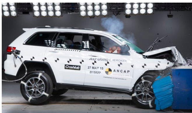
Frontal offset test at 64km/h
