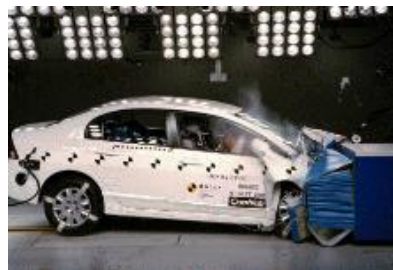
Offset crash test at 64km/hr
