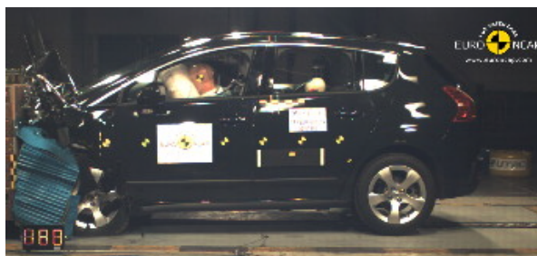
Offset crash test at 64km/h
