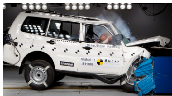
Offset crash test at 64km/h
