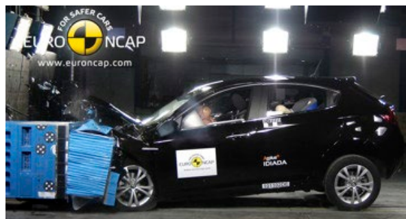
Offset crash test at 64km/h
