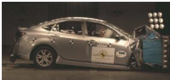
Offset crash test at 64km/hr
