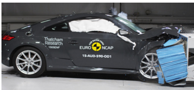
Frontal offset test at 64km/h
