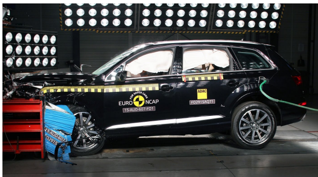
Frontal offset test at 64km/h
