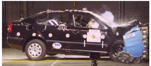
Offset crash test at 64km/hr
