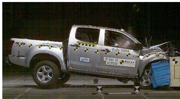
Frontal offset test at 64 km/h
