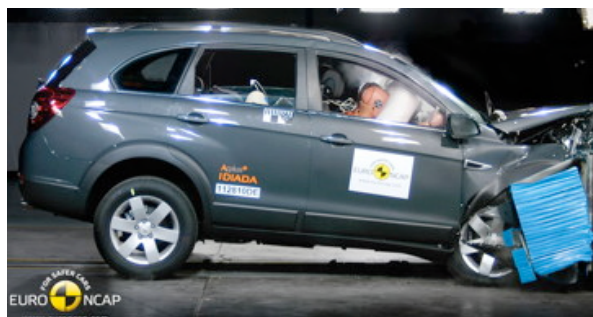
Offset crash test at 64km/h
