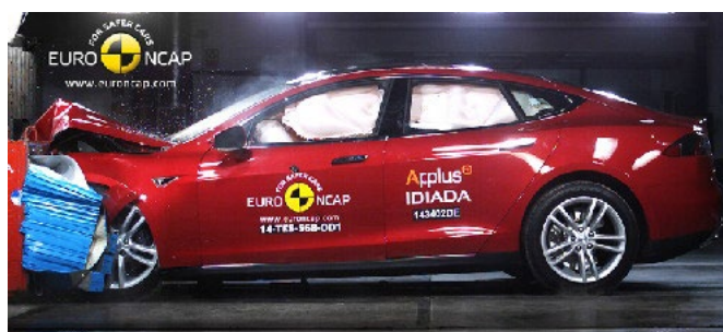
Frontal offset test at 64km/h
