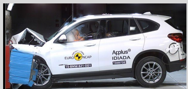
Frontal offset test at 64km/h
