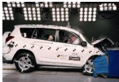
Offset crash test at 64km/hr
