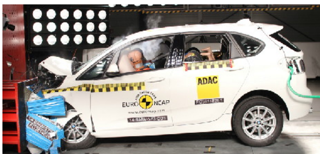
Frontal offset test at 64km/h (Euro NCAP)
