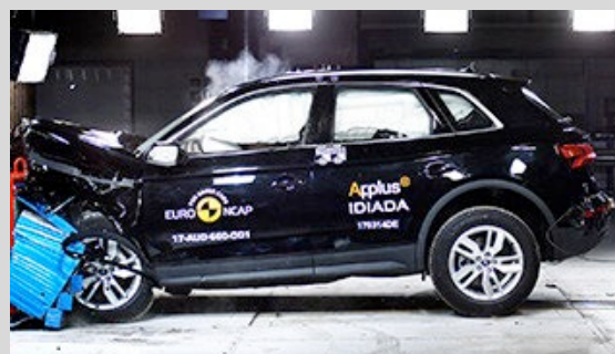
Frontal offset test at 64km/h
