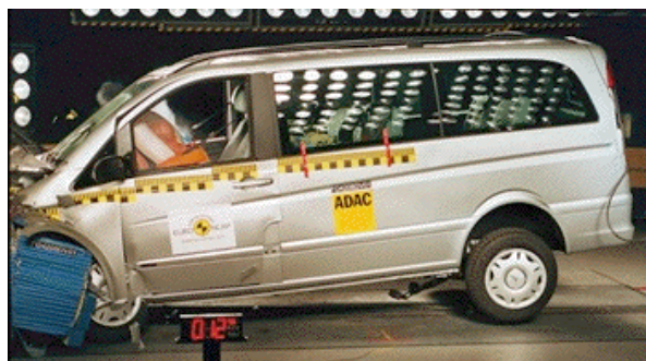
Offset crash test at 64km/h (Viano)
