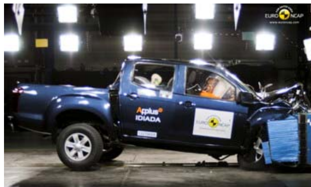
Frontal offset test at 64 km/h (Euro NCAP)
