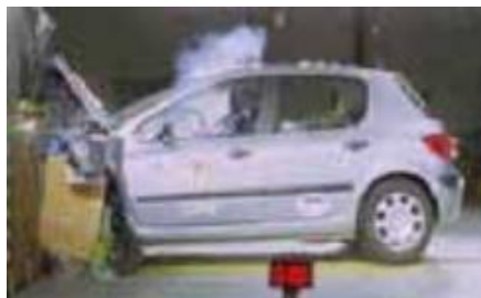
Offset crash test at 64km/hr
