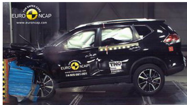
Frontal offset test at 64 km/h (Euro NCAP)
