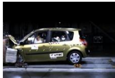
Offset crash test at 64km/hr
