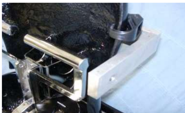
Figure 26: HPM back pan held by retaining strap.
