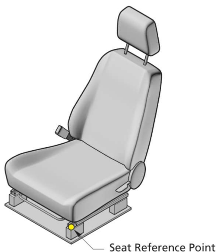
Figure 1: Definition of the Seat reference point.
