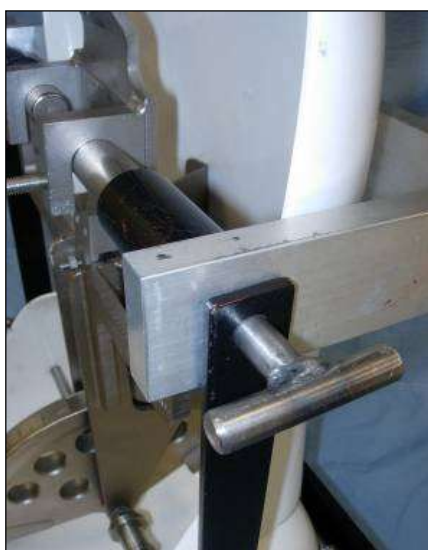
Figure 27: Weight hanger support pins inserted through weight hanger guide bars.
