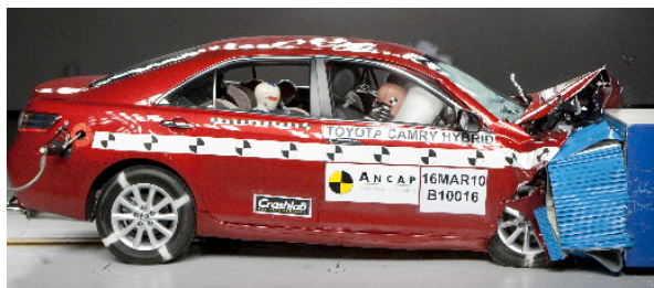
Offset crash test at 64km/h
