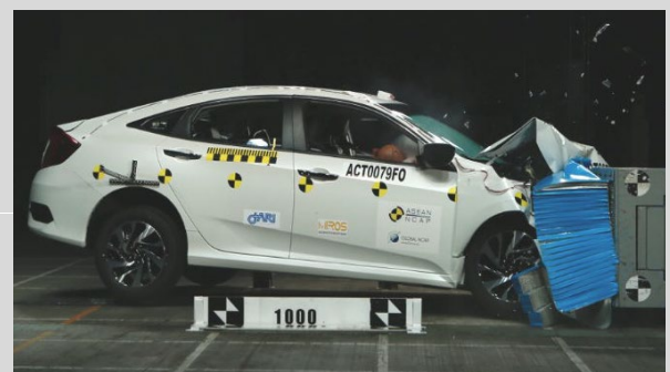
Frontal offset test at 64km/h (Honda Civic sedan)
