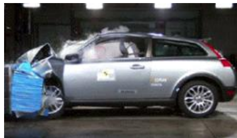
Offset crash test at 64km/hr
