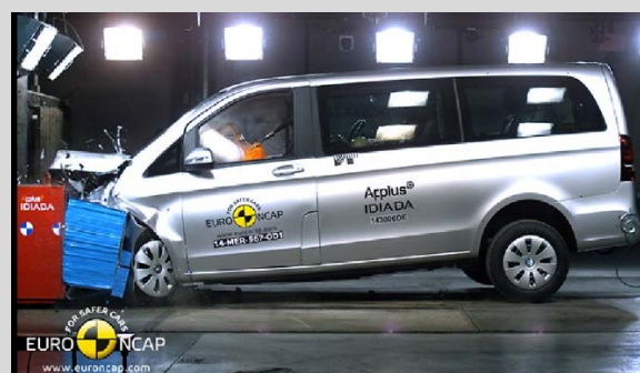
Frontal offset test at 56km/h (Mercedes-Benz V-Class)
