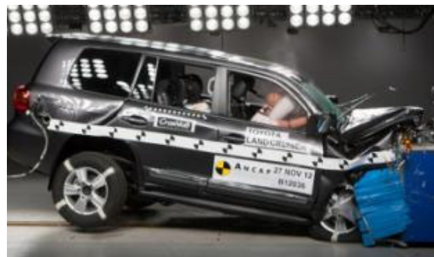
Frontal offset test at 64 km/h
