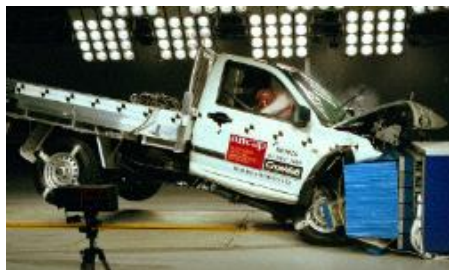
Offset crash test at 64km/hr
