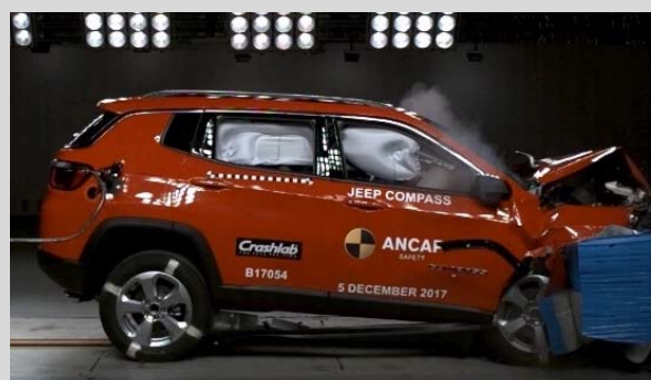
Frontal offset test at 64km/h
