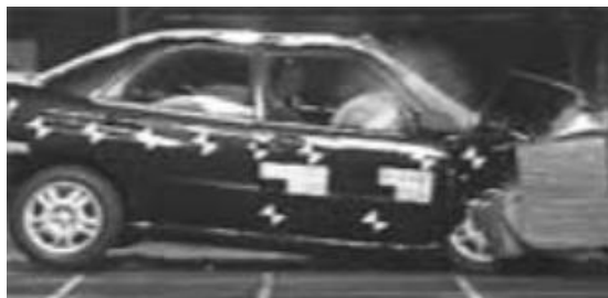
Offset crash test at 64km/hr
