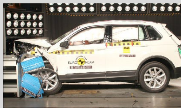
Frontal offset test at 64km/h
