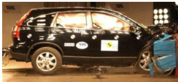
Offset crash test at 64km/hr
