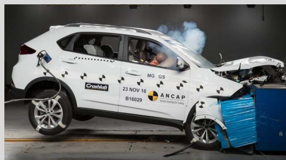
Frontal offset test at 64km/h
