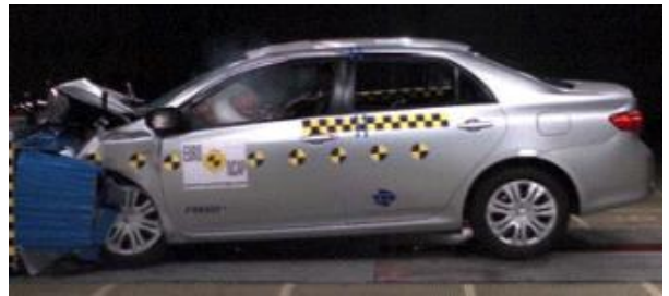
Offset crash test at 64km/hr
