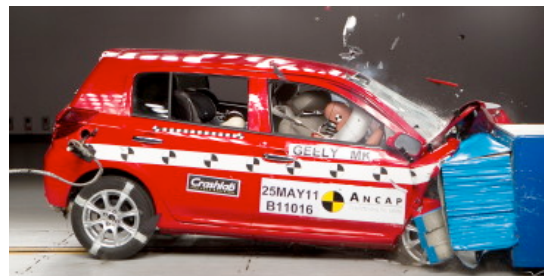
Offset crash test at 64km/h
