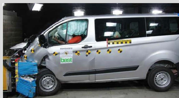
Frontal offset test at 56km/h
