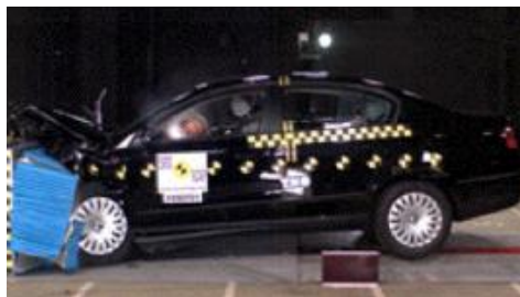
Offset crash test at 64km/hr
