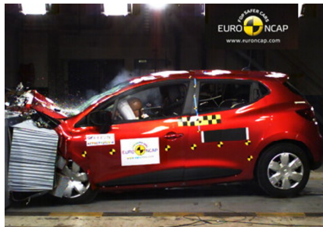
Frontal offset test at 64 km/h (Euro NCAP)
