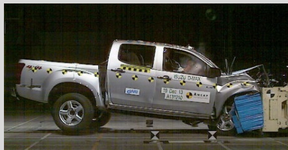
Frontal offset test at 64km/h (Isuzu D-Max)
